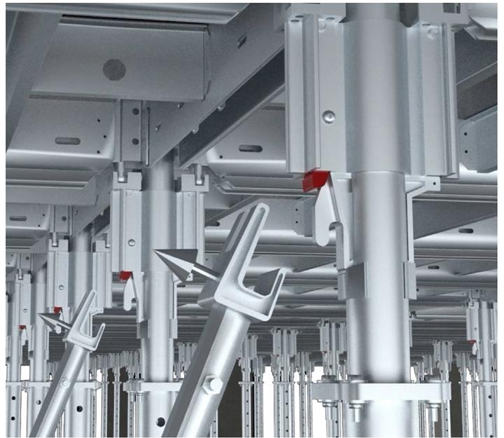
Featuring engineered Drop Heads with a rigid interlocking system, the props ensure enhanced safety by preventing tipping during erection. The integrated Cantilever System offers a secure working platform around the slab perimeter, while the Drop Head allows early panel removal without disturbing the props—ensuring effective back-propping remains in place.
